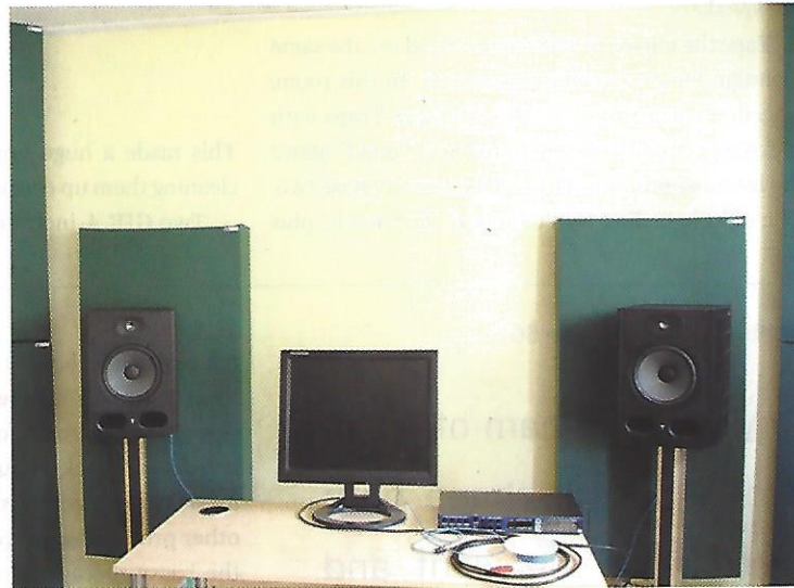
Fig. 4. Placing GIK 244 bass traps behind the speakers cleans up our low mids a great deal.
