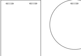
Drill holes in wall correct distance apart from centre of each sawtooth hanger. Ensure correct plugs and screws are used for wall type.
